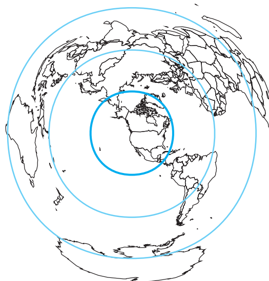
Fig. 2. Azimuthal equidistant projection centered at Seattle, Washington. Circles away from Seattle have an interval of 5000 km (3120 mi).
