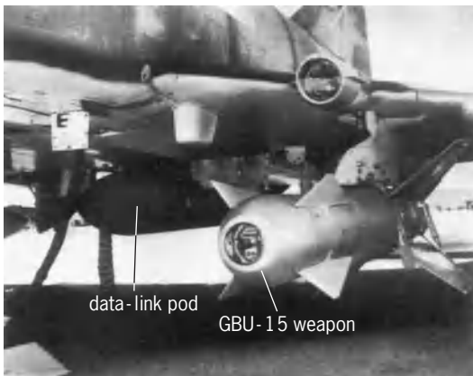
Fig. 1. GBU-15 with data link system, mounted on F-4 Phantom II fighter. (Hughes Aircraft Co.)
