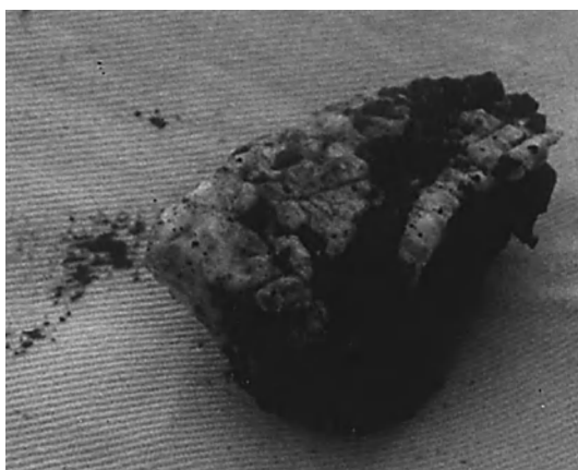
Methane hydrate core sample taken from the Costa Rica margin slope sediments about 200 m below the sea floor.
