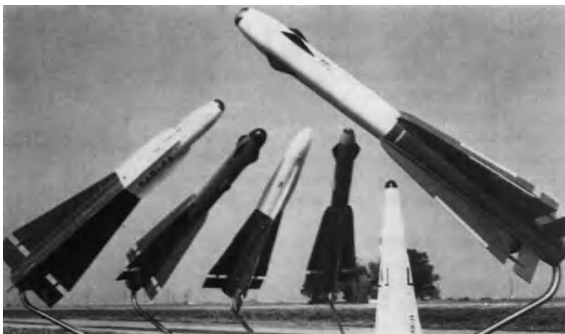
Fig. 6. Falcon air-to-air missile family, including missiles with infrared and radar guidance, and high-explosive and nuclear warheads. (Hughes Aircraft Co.)
