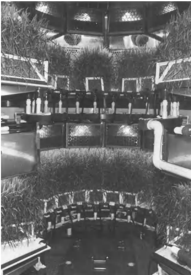
Fig. 2. Wheat grown under artificial lighting by using the nutrient film technique in the Biomass Production Chamber at the Kennedy Space Center. (NASA).
