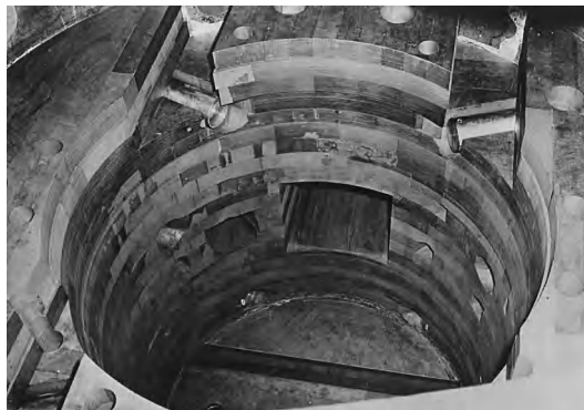
Fig. 3. Graphite reflector for a test reactor.
