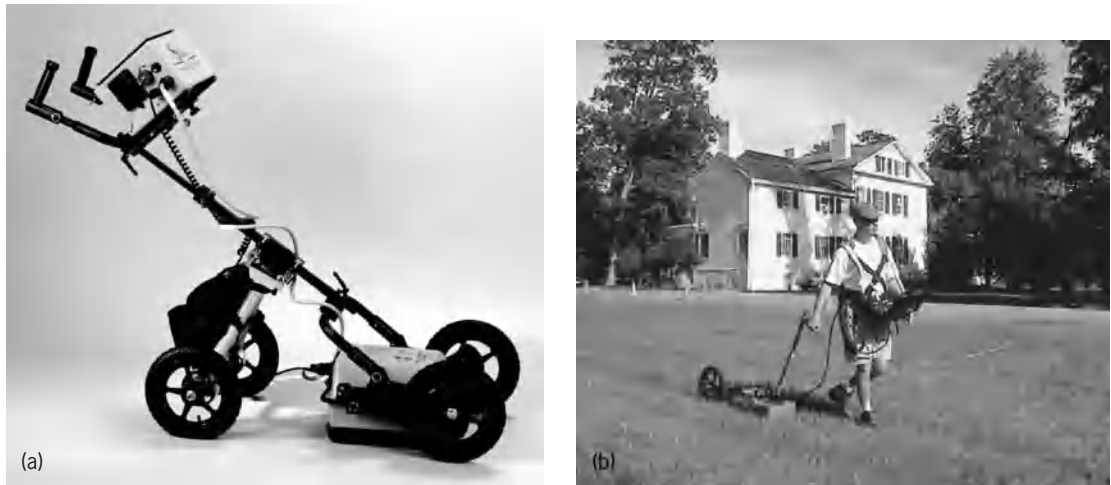
Fig. 1. Ground-penetrating radar equipment. (a) Portable equipment with 500-MHz antenna and controller that displays scrolling vertical slices of the soil in real time (USRADAR). (b) Portable equipment with 400-MHz antenna being used in archeological survey at Franklin D. Roosevelt's Hyde Park Estate in New York (Geological Survey Systems, Inc.).
