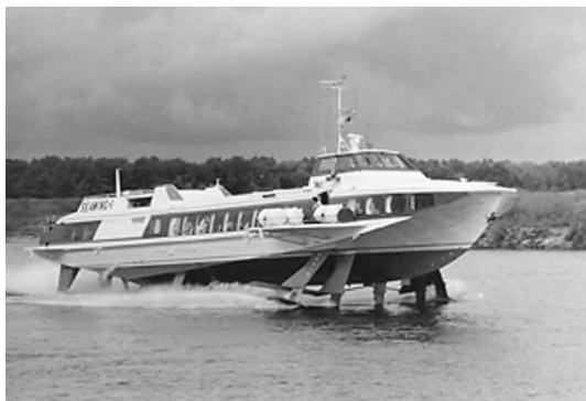
Fig. 4. Russian hydrofoil in Katran Class. (Volga Shipyard)
