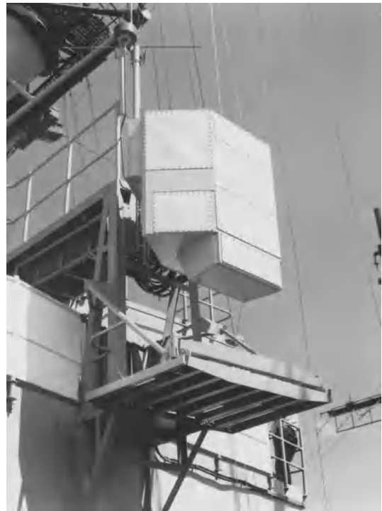
Fig. 8. Antenna for shipborne deception ECM system mounted on vessel's superstructure. (Hughes Aircraft Co.)
