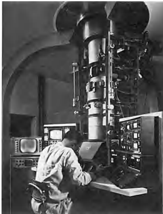
Fig. 5. TV image intensification system for the electron microscope. (Radio Corporation of America)
