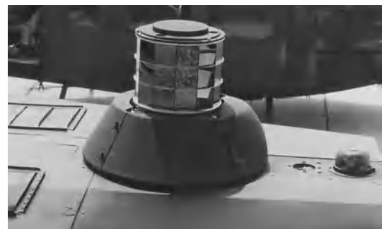
Fig. 5. Transmitter of infrared countermeasures system, providing 360° protection, mounted atop fuselage of UH-1H utility helicopter. (Sanders Associates)
