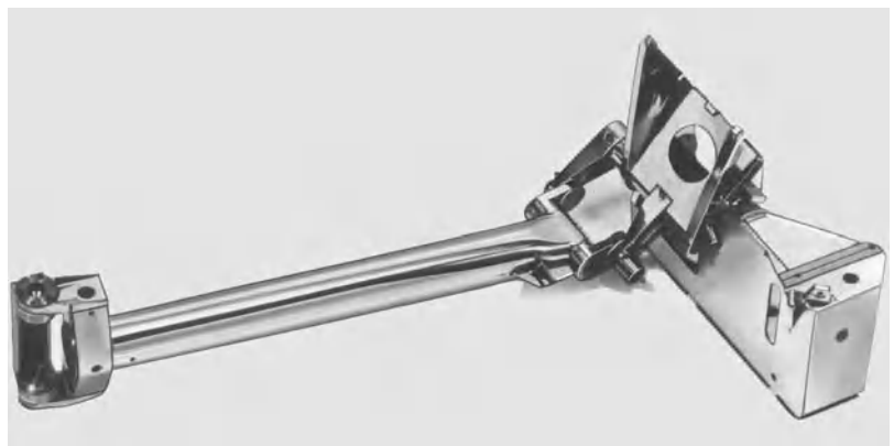
Fig. 4. Planetary boom of the Mariner 2 spacecraft.
