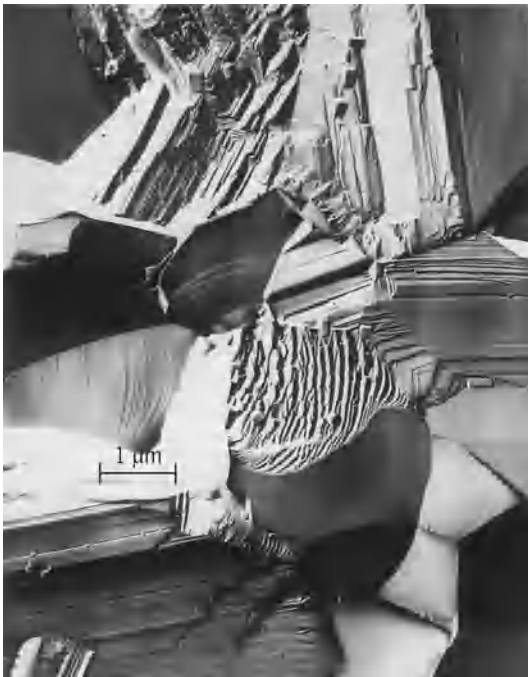
Fig. 17. Replica of a fractured surface of a magnesia ceramic. (Courtesy of T. T. Sheng)
