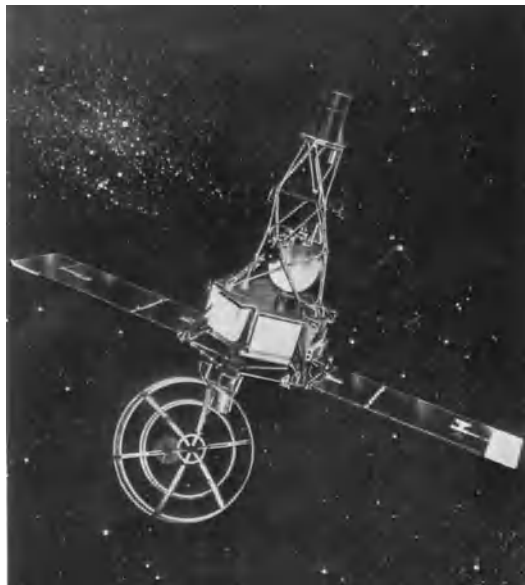
Fig. 3. Flight configuration of Mariner 2 spacecraft.
