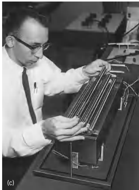
Fig. 1. Calculable capacitor. (a) Cross section of general cylindrical capacitor with four segments. (b) Cross section of symmetrical capacitor with cylindrical electrodes. (c) Calculable capacitor used in absolute determination of the ohm. (U.S. National Institute of Standards and Technology)
