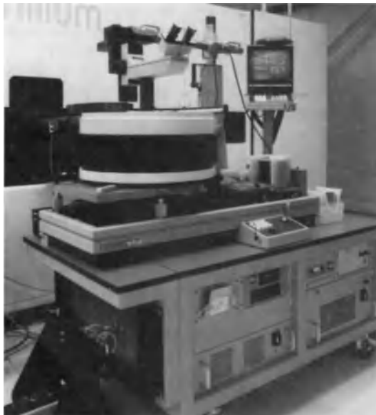
Automatic test equipment for testing microelectronic devices. (Rockwell International)
