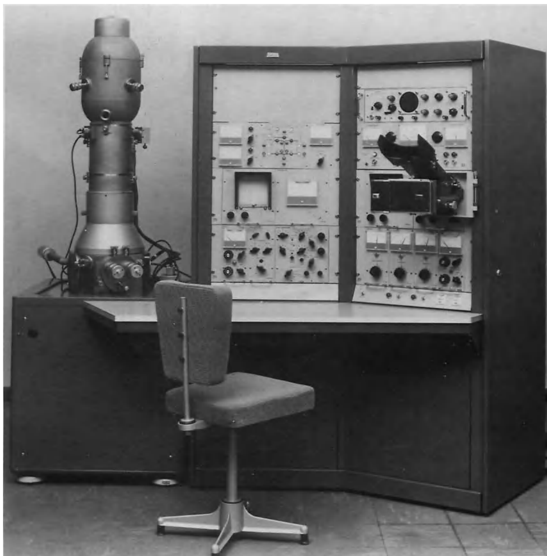
Fig. 6. Megavolt electron microscope at U. S. Steel research laboratory at Monroeville, Pennsylvania. ( Radio Corporation of America )
