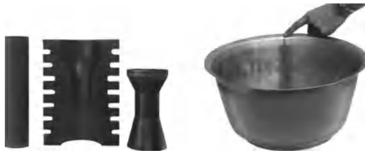
Fig. 2. Typical metal shapes produced by explosive forming. Note weld in bowl. (National Northern Corp.)
