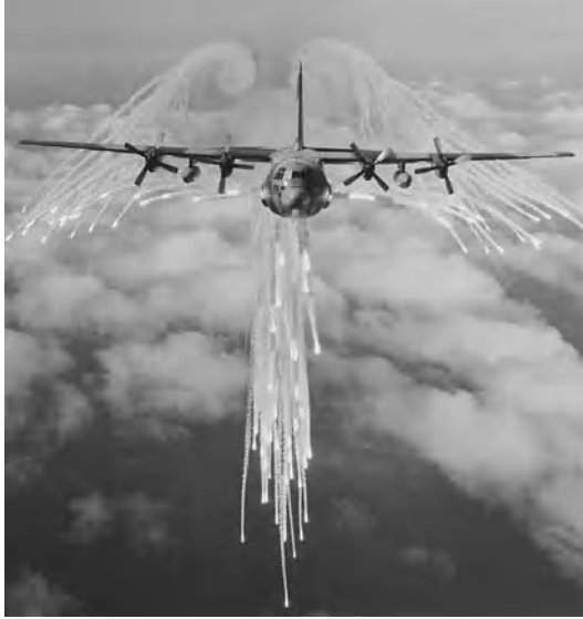
Fig. 4. Countermeasures-dispensing system aboard an air transport used in humanitarian relief efforts ejecting flares to foil attacks by ground-launched infrared guided missiles. (Lockheed Aircraft Service Co.)
