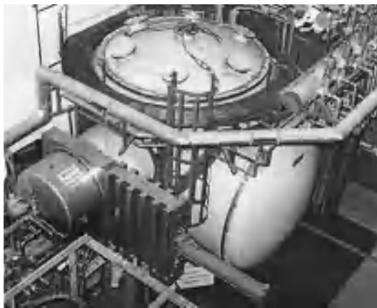
Fig. 2. Large "sunspot chamber" for Earth orbital and deep-space simulations of spacecraft, located at the Marshall Space Flight Center. (NASA)
