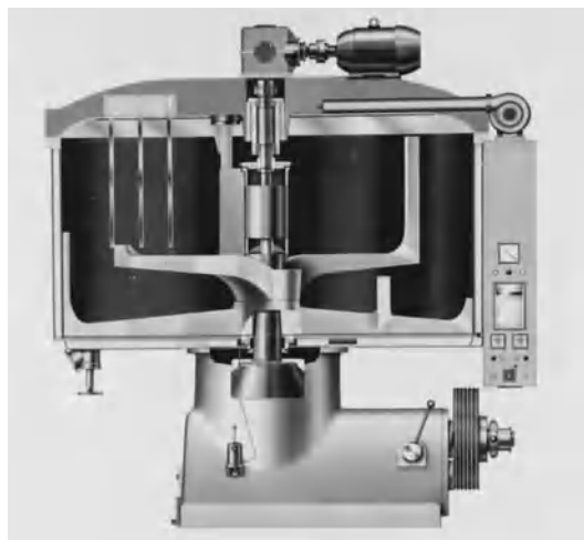
Fig. 3. Modern rotary conche. (Petzholdt, Frankfurt, Germany)
