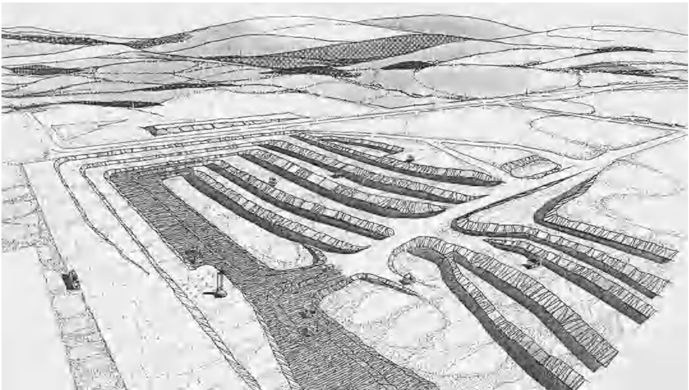
Fig. 1. Diagram of a terrace pit coal mine, showing terrace pit stripping and reclamation. (After U.S. Department of Energy, The Development of Optimal Terrace Pit Coal Mine Systems , DOE Rep. FE/10023-1, January 1971)
