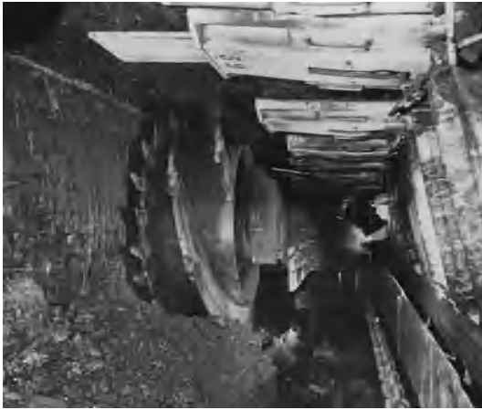
Fig. 16. Longwall shearer and hydraulic roof support.
