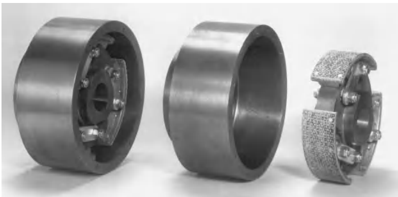
Fig. 3. Internal-expanding centrifugal-acting rim clutch. (Hilliard Corp.)
