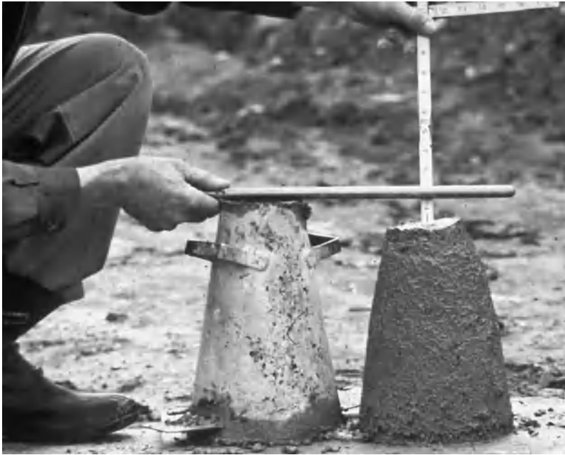
Fig. 2. Concrete slump test with a slump of 1.5 in., typical for pavement work. (Portland Cement Association)
