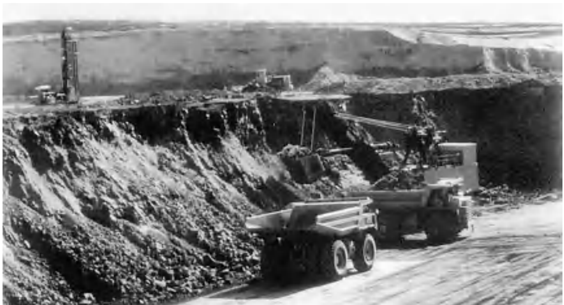
Fig. 5. Power shovel loading coal trucks.
