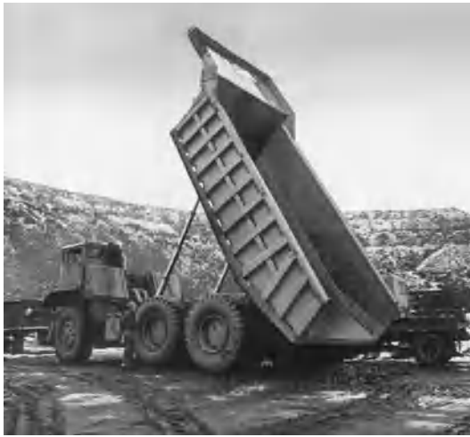
Fig. 6. A 100-ton (90-metric-ton) rear-dump truck.
