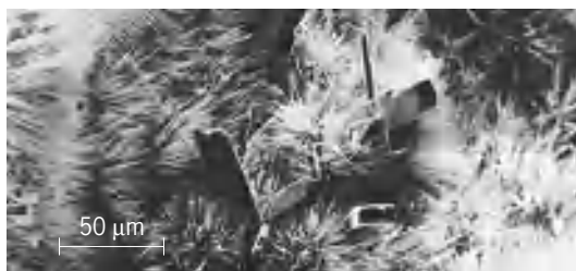
Micrograph of a portland cement formulation cured at 390–450°F (200–230°C) for 72 h; gypsum and xonotlite crystals are growing into a cavity.
