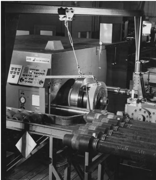
Fig. 4. Inertia welding machine for oil drill pipe sections.
