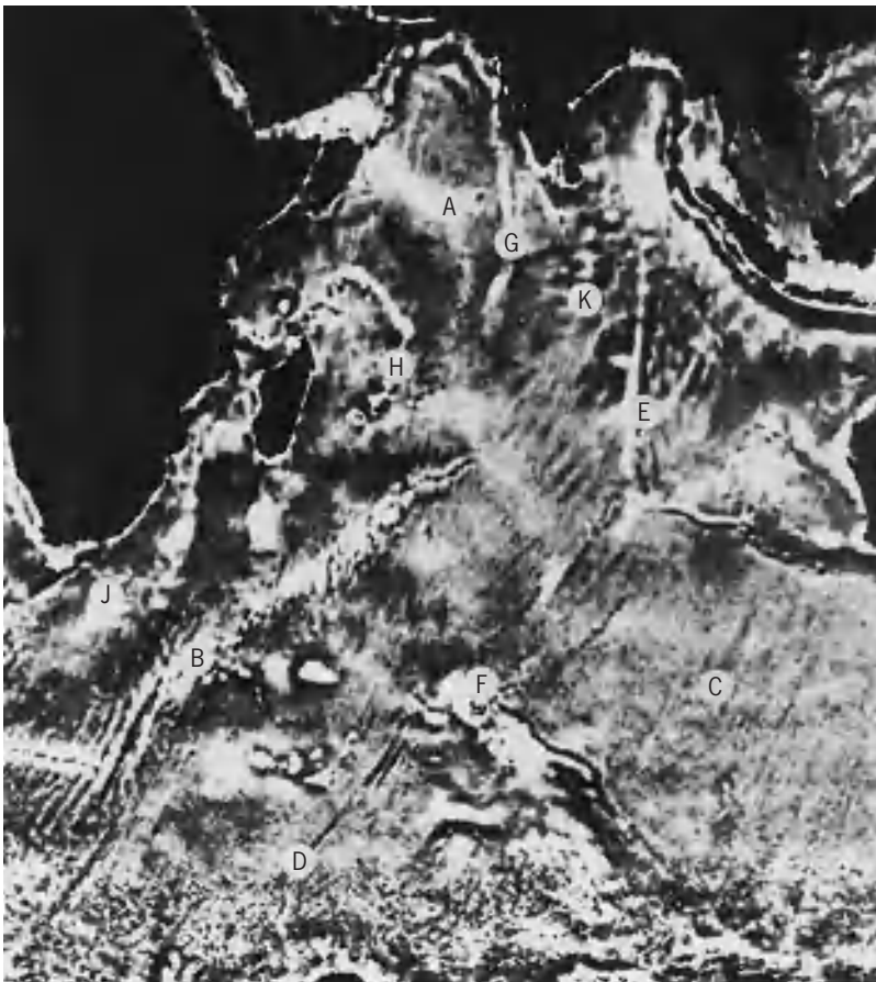
Fig. 8. Geotectonic image of the Indian Ocean as reflected in the satellite-derived gravity field of the region. A few specific structural features are identified as follows: Spreading centers: A, Carlsberg Ridge; B, Southwest Indian Ridge; C, Southeast Indian Ridge. Fracture zones: D, Indian-Antarctic; E, Ninety East Ridge (tentatively identified as a fracture zone). Plateaus: F, Kerguelen; G, Chagos-Lacadive; H, Mascarene; J, Agulhas. Zone of intraplate deformation, K. (W. Haxby, Lamont-Doherty Geological Observatory of Columbia University)
