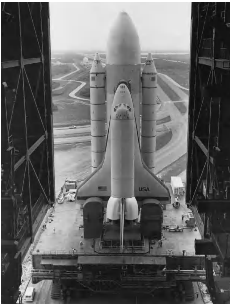
Fig. 9. Fully assembled space shuttle on the mobile launcher leaving the Vehicle Assembly Building. (NASA)
