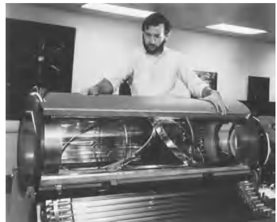
Fig. 4. High-power laser amplifier stage, with a 30-cm (1-ft) aperture, using liquid-cooled slabs of neodymium:glass. (Lawrence Livermore National Laboratory)
