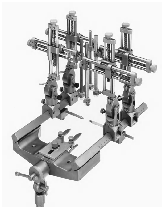
Fig. 2. Stereotaxic instrument designed to allow precise placement of electrodes into brain structures. Note the four electrode carriers positioned above the area where the animal's head would be placed. (Kopf Instrument Co.)
