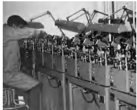
Fig. 1. Automatic cupping machines for the manufacture of jewel bearings. (Bulova Watch Co.)
