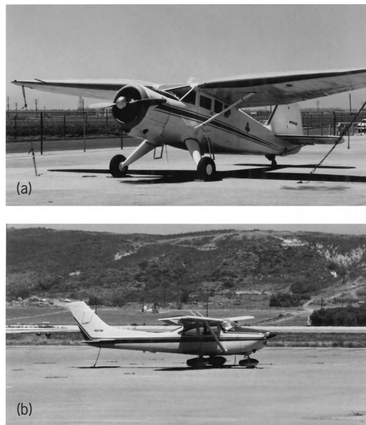
Fig. 1. Landing gear arrangements. (a) Tail-wheel arrangement. (b) Tricycle arrangement.
