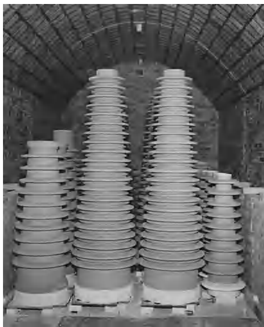
Fig. 3. Interior of periodic kiln, with electrical porcelain insulators for firing. (Swindell-Dressler, Inc.)
