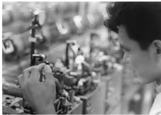
Fig. 3. Technician shown operating an automatic cupping machine. (Bulova Watch Co.)
