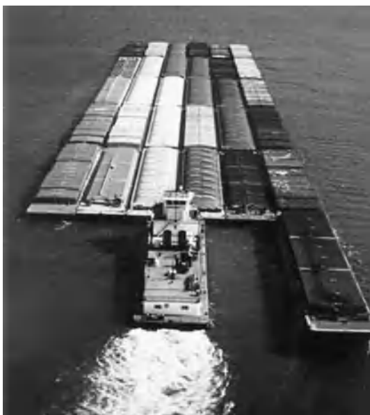
Fig. 3. Inland tow, consisting of open and closed dry cargo barges, being pushed ahead by a towboat. ( The American Waterways Operators )
