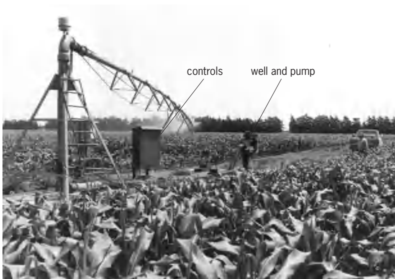
Fig. 4. Center-pivot irrigation system irrigating corn. A single unit can water as much as 500 acres (200 hectares) or more. (Eastern Iowa Light and Power Cooperative)
