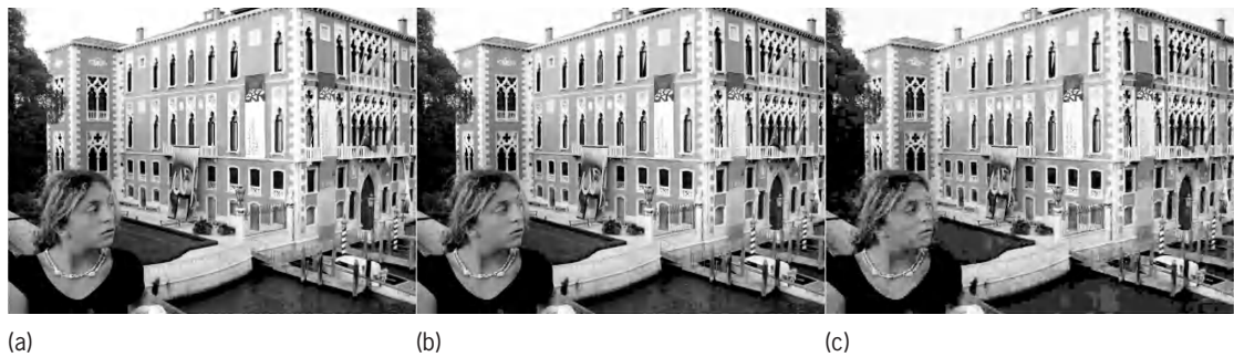
Fig. 3. Example of compression. (a) Original 1024 \times 768 pixel image, at 3.3 bits per pixel (bpp), typical of the compression provided by digital cameras. (b) Compressed version of the original image using JPEG compression, at 0.7 bpp. There is little visual degradation, yet the file size is over 4 times smaller. (c) Further compressing the image to 0.4 bpp; noticeable degradation has occurred with this lossy algorithm.
