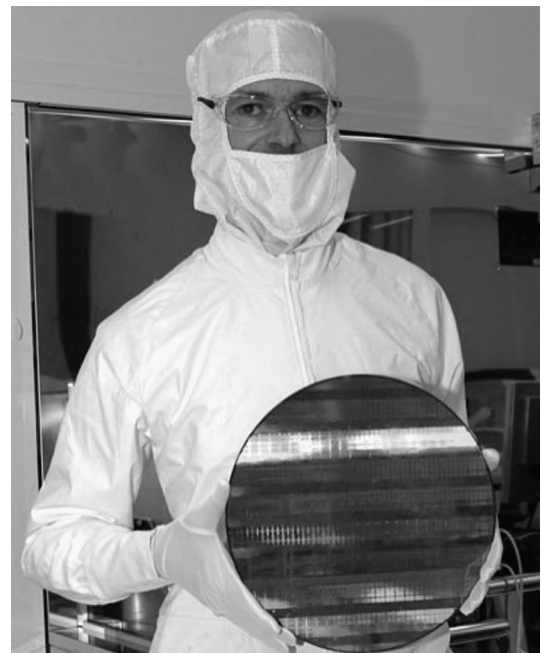
Fig. 7. Person with lint-free garments in a vertical laminar-flow clean room for integrated-circuit fabrication with 300-mm (12-in.) wafer. (Personnel do not handle wafers in this manner. This was done just for the photograph.) ( Intel Corp. )
