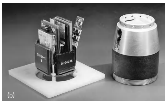
Fig. 6. Strap-down inertial navigation systems. (a) Mock-up of system based on laser gyro technology. The three laser gyros, hermetically sealed, are on the left (Honeywell). (b) 130-cm 3 (8-in. 3 ) system that uses silicon MEMS technology (Draper Laboratory).
