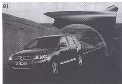
Figure 35. Use of integral skin foams and RIM materials A) Fender of the VW Touareg; B) Snowmobile
