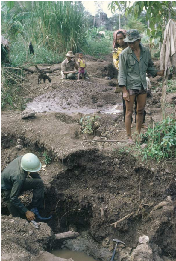
Figure 5 Eluvial workings in weathered (decomposed) basalt above basalt lava (Pailin, Cambodia). © Alan Jobbins.
