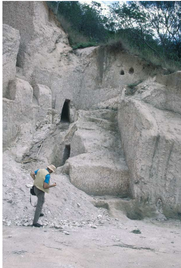
Figure 6 Workings in granite with cross-cutting pegmatite, which is a source of aquamarine and chrysoberyl (River Marambio Baia, Minas Gerais, Brazil). © Alan Jobbins.
