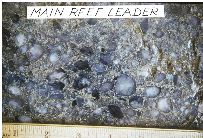
Figure 9 A typical specimen of Witwatersrand gold ore from South Africa. Pyrite and minor gold in the groundmass supporting well-rounded, unmineralized quartz pebbles, 25 cm across. Photo: GR Davis.
