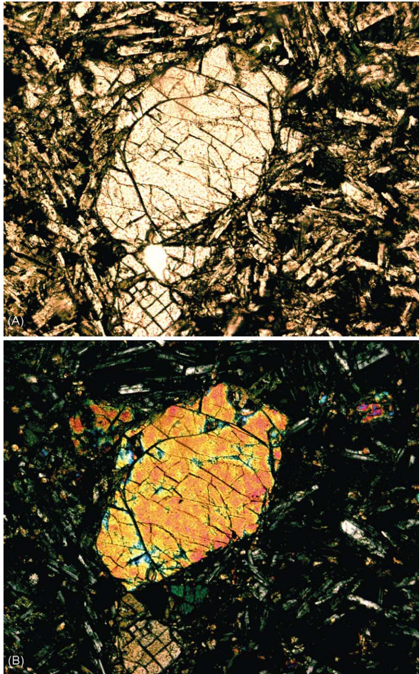
Figure 2 Basalt (from Melbourne, Victoria) seen in thin section through a polarizing microscope showing a euhedral phenocryst of olivine in plane polarized light (A), and with crossed polars (B).
