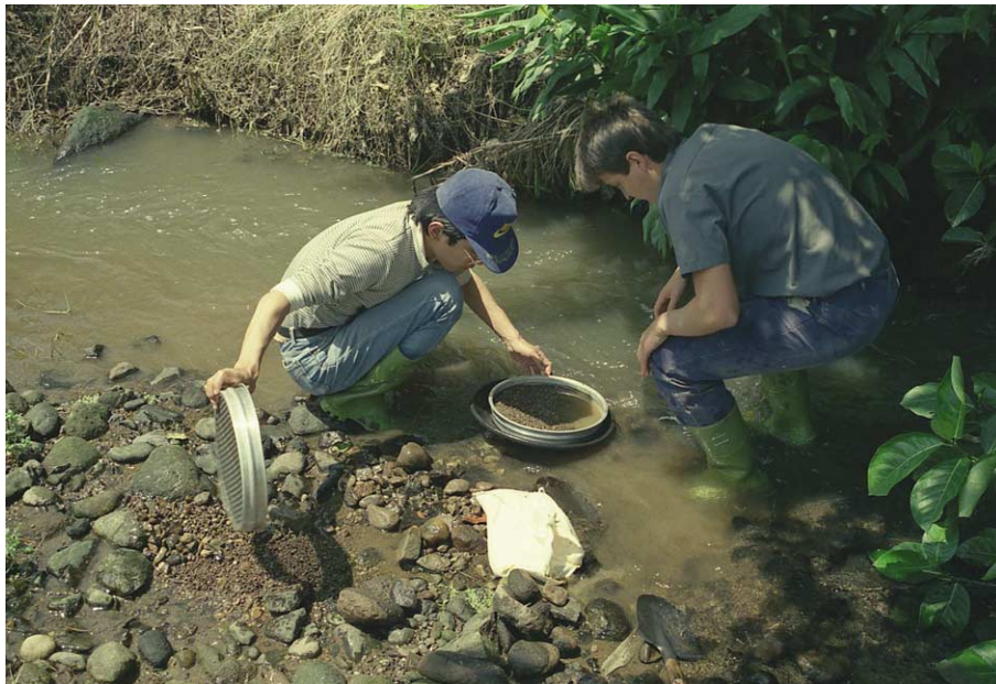
Figure 3 Geochemical sampling in eastern Taiwan. Sediments are dug from the creek bed, sieved to remove the largest pieces, and the finer fraction is bagged and sent to a laboratory for chemical analysis.
