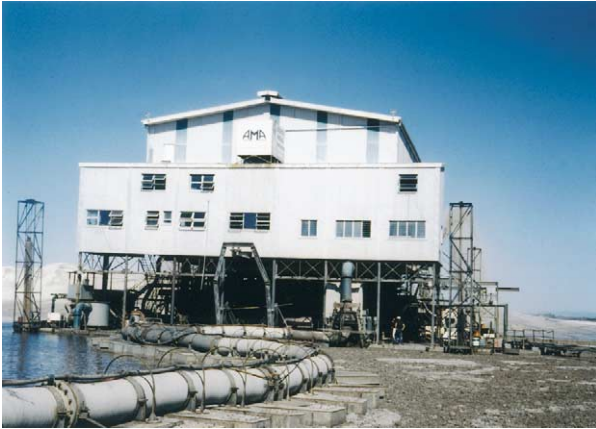
Figure 8 A dredge working on a deposit of rutile and zircon on Stradbroke Island off the Queensland coast. Such large and complex installations require capitalization running into millions of dollars. Photograph by GJH McCall.
