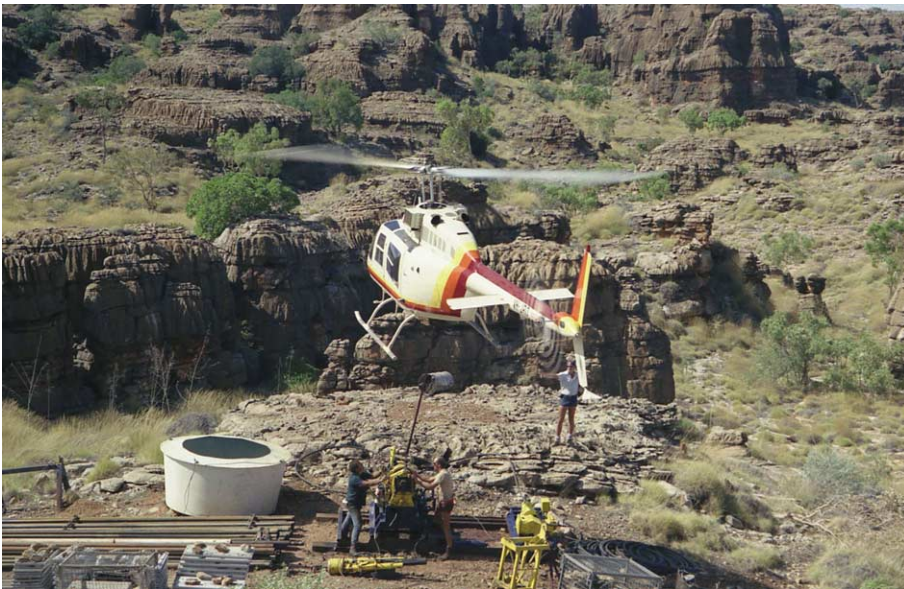
Figure 6 A helicopter being used to move a diamond drilling rig in the Kimberley region of Western Australia. The helicopter allows the drill to be positioned with minimal disturbance and environmental damage.
