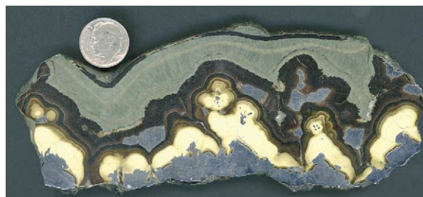
Figure 1 Banded, crustiform sphalerite (ZnS, yellow to brown) and marcasite (FeS 2 , green) with later pore-filling, cross-cutting galena (PbS, grey) in polished slab of hydrothermal ore from Olkusz mine, Silesian–Cracovian lead–zinc district, Poland. US 10 cent coin for scale.
