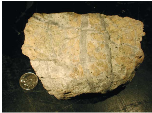
Figure 3 Porphyry Cu-Mo ore showing cross-cutting silica veins, from Gross Peak pit, Ithaca Peak (Mineral Park) mine, Arizona. US 10cent coin for scale.
