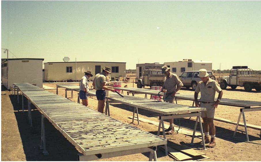
Figure 7 Examining trays of drill core from the Eloise copper–gold deposit in western Queensland, Australia. Diamond drilling techniques are used, which allows deep holes to be drilled, and the core recovered allows detailed geological examination.
