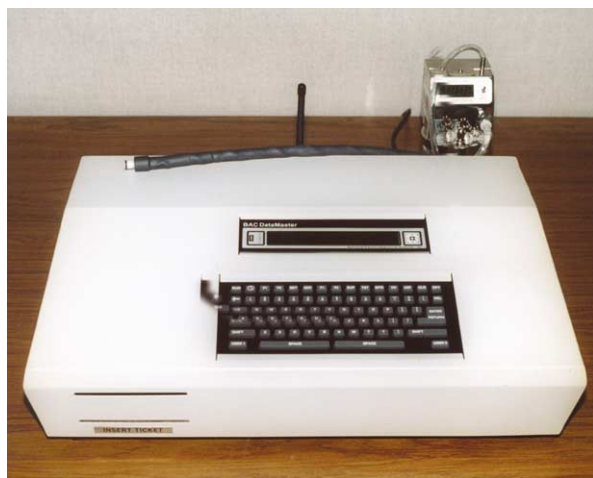
Figure 3 The BAC Datamaster breath-testing instrument showing a wet-bath control simulator standard device attached.
