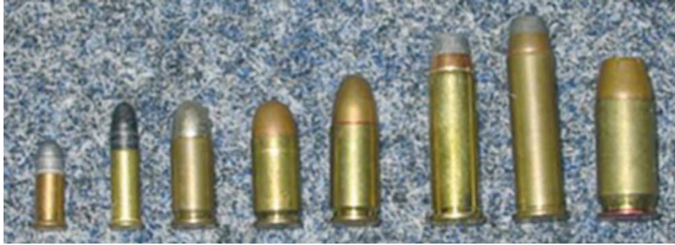
Figure 8 Handgun cartridges (from left to right): 0.22 short, 0.22 long rifle, 7.65 mm, 9 mm short, 9 mm Parabellum, 0.38 Special, 0.357, and 0.45.
