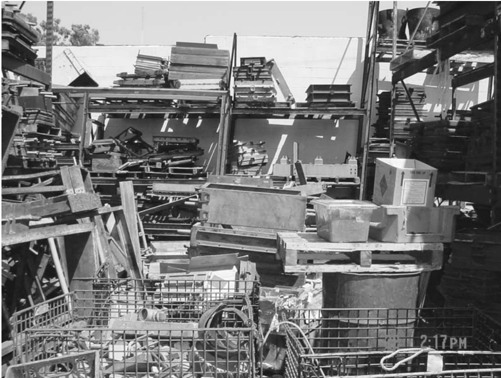
Fig. 2 In this messy plant, the workers waste close to 20% of their time looking for items and scavenging for parts and tools, also wasting the plant energy.
