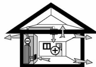
Fig. 11 HVAC equipment effect on building pressure differences.
