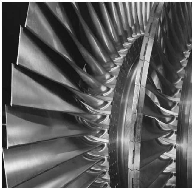
Fig. 9 Low pressure rotor. (Courtesy of Siemens AG.)
