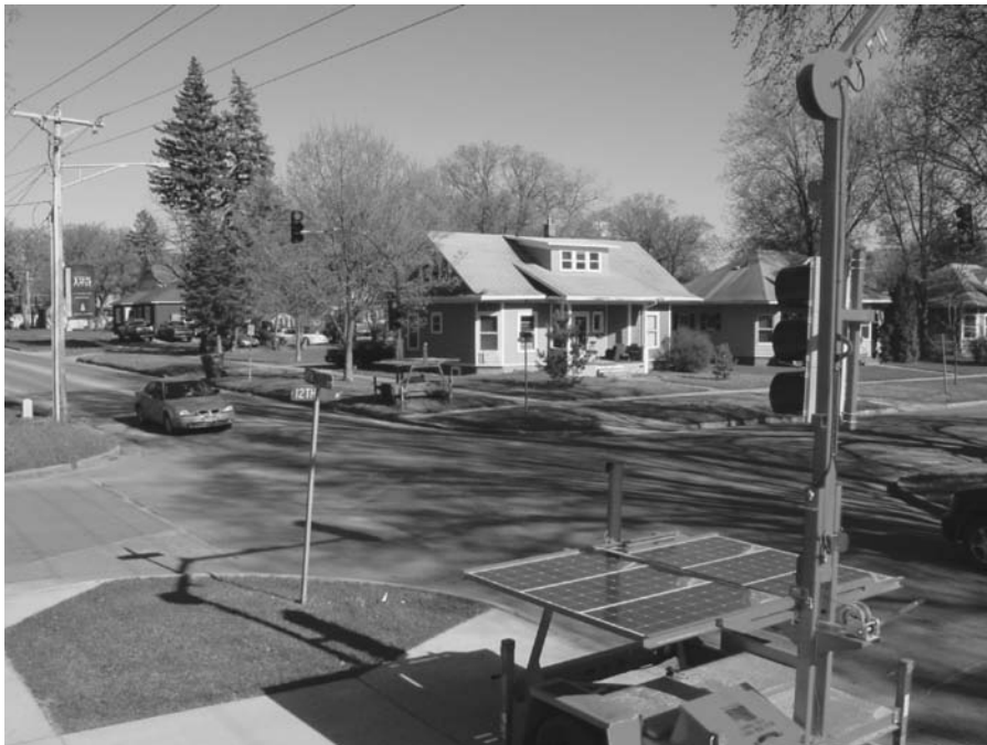
Fig. 12 Traffic signaling applications: a temporary stoplight in a construction zone in Brookings, South Dakota (Photo by Michael Ropp).
