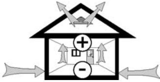
Fig. 12 Stack effect on building pressure differences.
