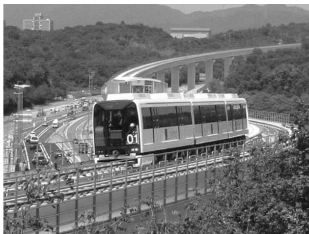
Fig. 7 Super-quiet low-speed (100 kph) “Linimo” maglev in commercial operation outside Nagoya, Japan.
