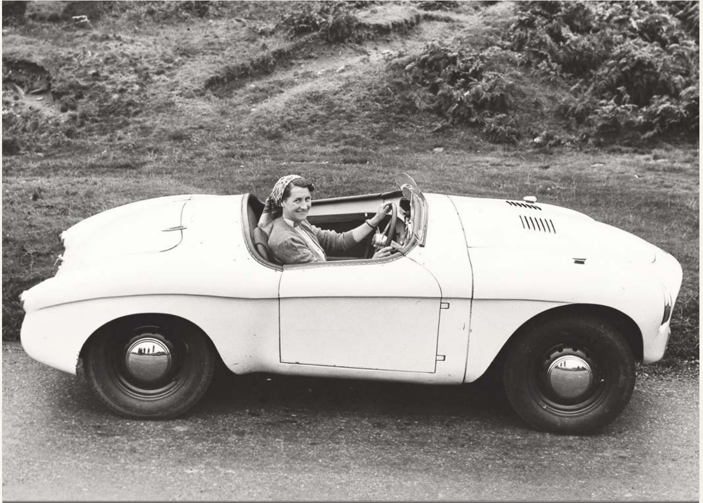
Fiberglass body panels meant that the sporty Jupiter R4 could be produced cheaply, but it came too late to save the Yorkshire-based company.
