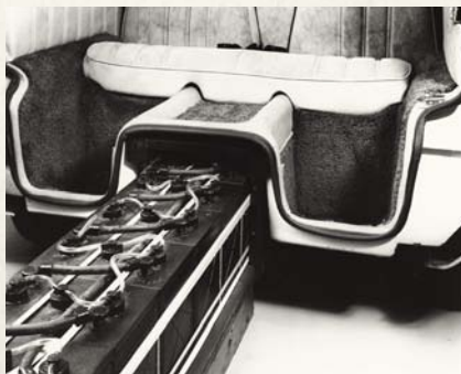
The pull-out battery pack was inserted along the center of the car's underside.
