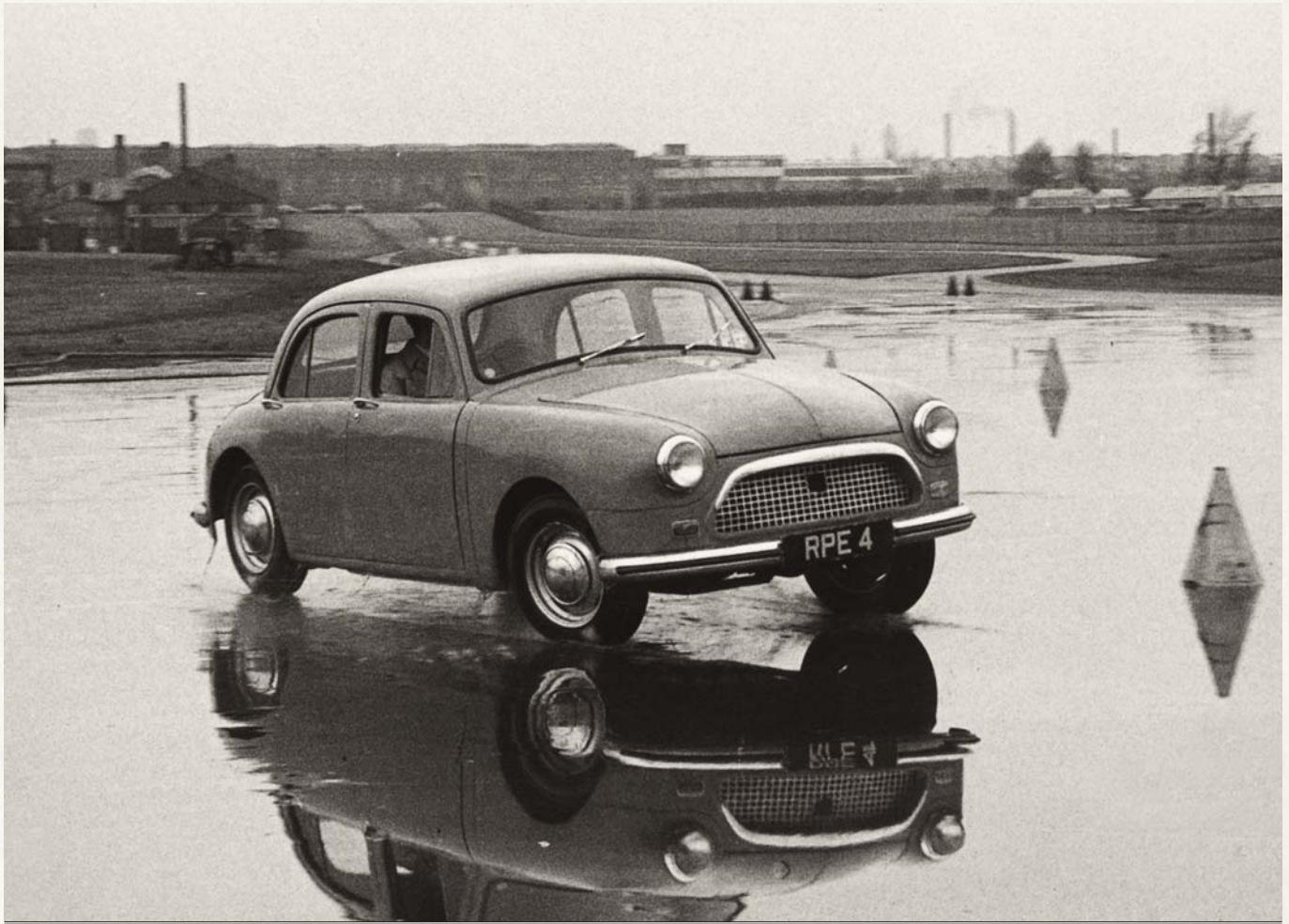
Slippery conditions were just the kind of thing the Ferguson R4 sought to conquer, with the extra road adhesion supplied by four-wheel drive.
