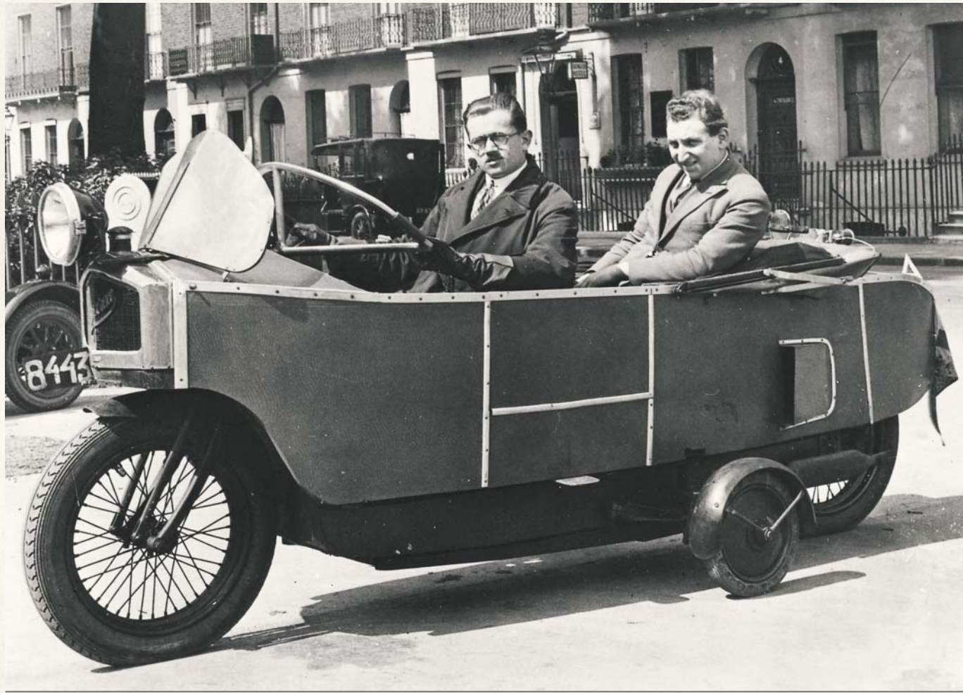
The Monotrace was nominally a two-wheeler "car," although it had drop-down stabilizer wheels for stationary moments.
