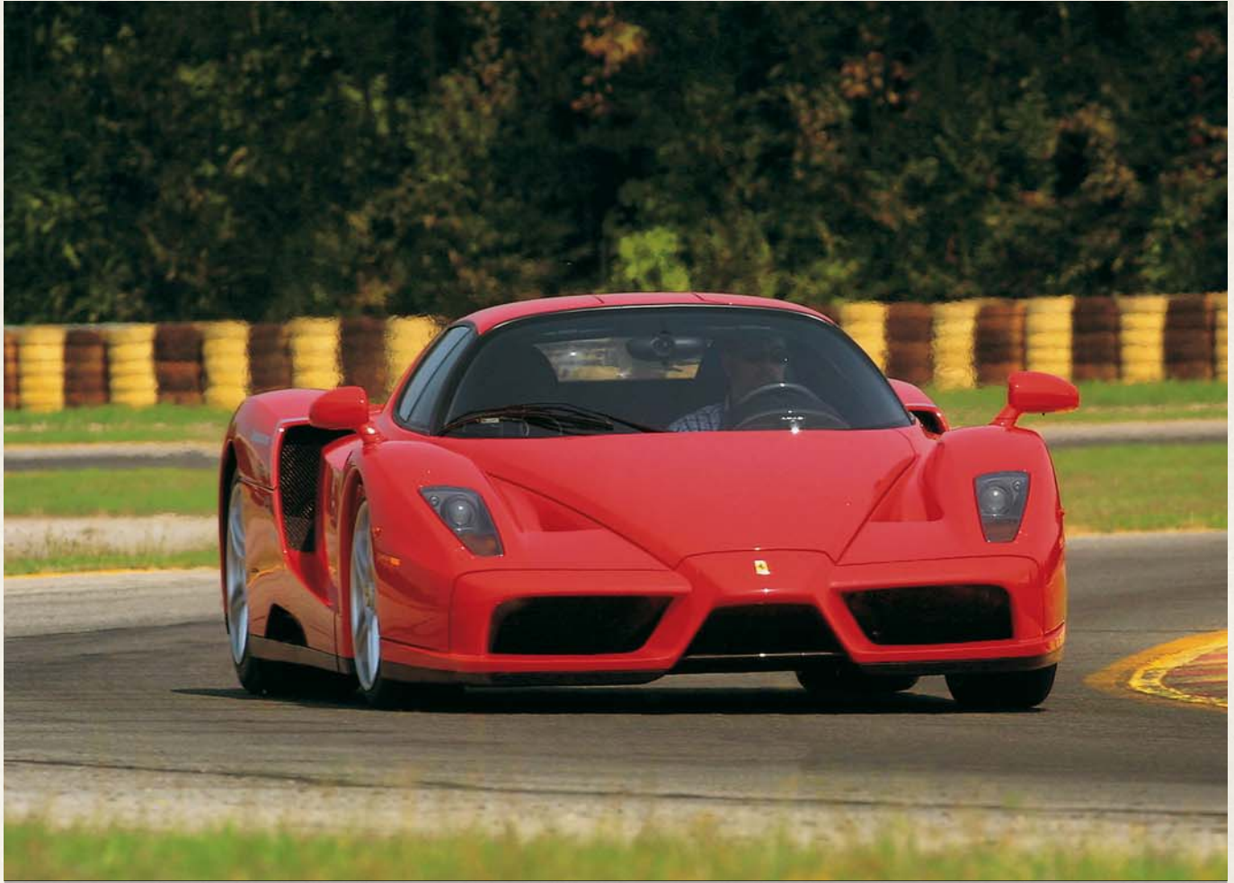
Active aerodynamics, a body/chassis made of carbon fiber, and carbon-ceramic brakes featured in this stunning tribute to the founder of Ferrari.
