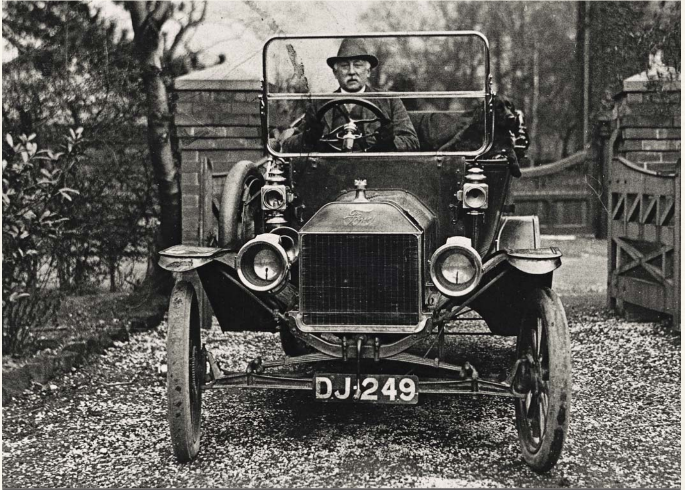
The Model T always boasted a high-ground clearance among its sturdy attributes, making it well-suited to the state of roads in 1920s America.
