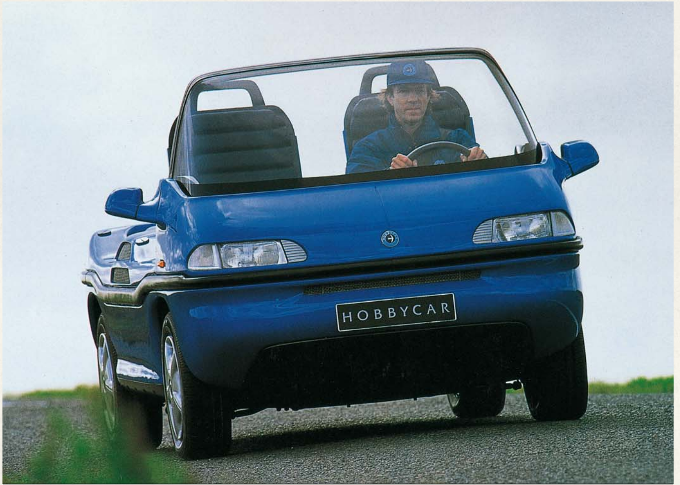
With its four-wheel drive, rugged construction, and adjustable height, the Hobbycar was meant to be as useful on road as it was enjoyable in water.
