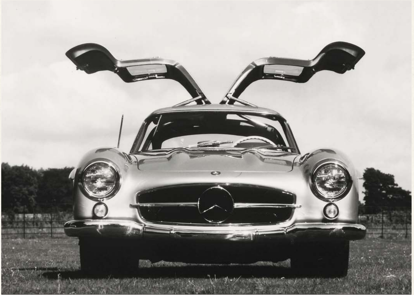
The novel “gull-wing” doors were there to preserve chassis rigidity rather than impress the neighbors!
