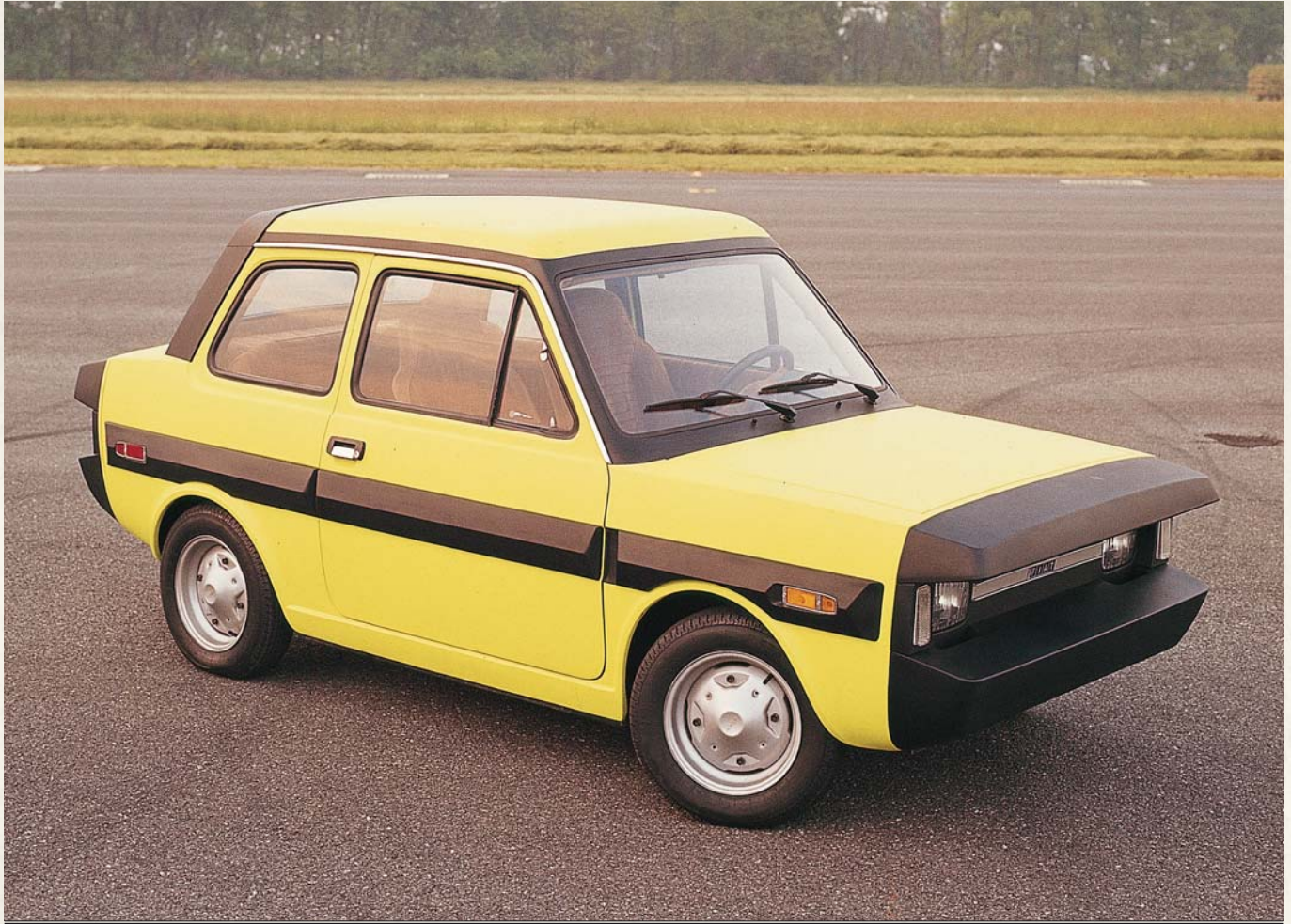
The prominent black plastic “bumpers” were meant to be kind to pedestrians, while ESV occupants enjoyed a cabin fortified against impacts.
