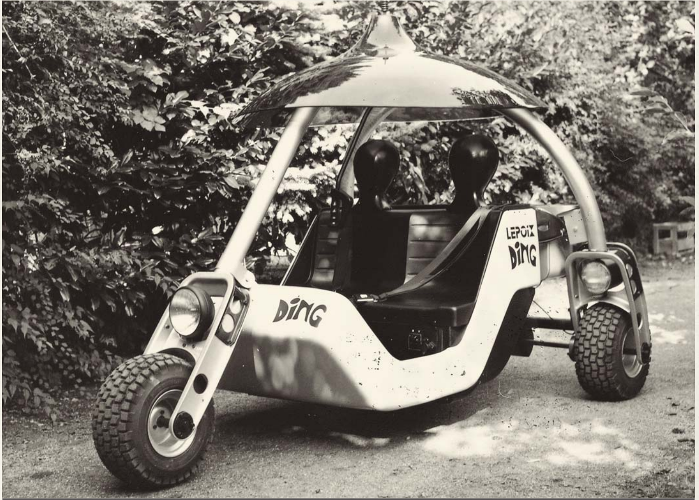
It almost defies description, but the Lepoix Ding, with its battery power, really could be driven—by someone standing at the back using a tiller.
