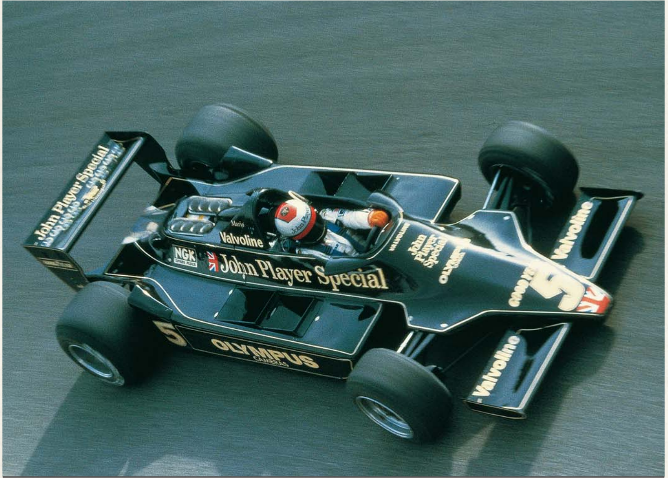
The entire body of the 79 was used as a vacuum to suck the car down on to the racetrack; this “Black Beauty” proved dominant on the F1 grid.
