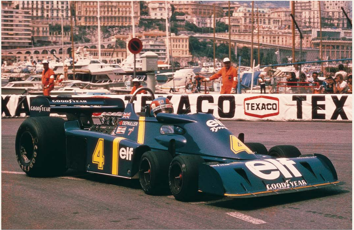
Patrick Depailler putting the Tyrrell P34 through its paces on the Monaco Grand Prix circuit; note the small “window” for placing the six wheels.
