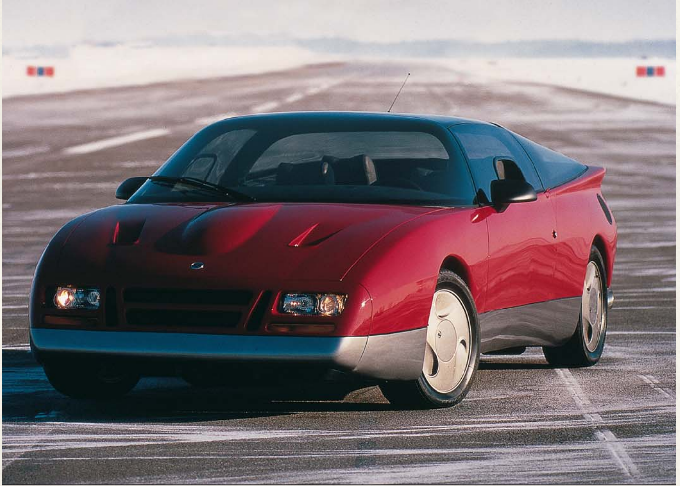
With admirable Swedish logic, Saab used the EV-1 as the opportunity to create an advanced but fully working research car using 900 Turbo parts.
