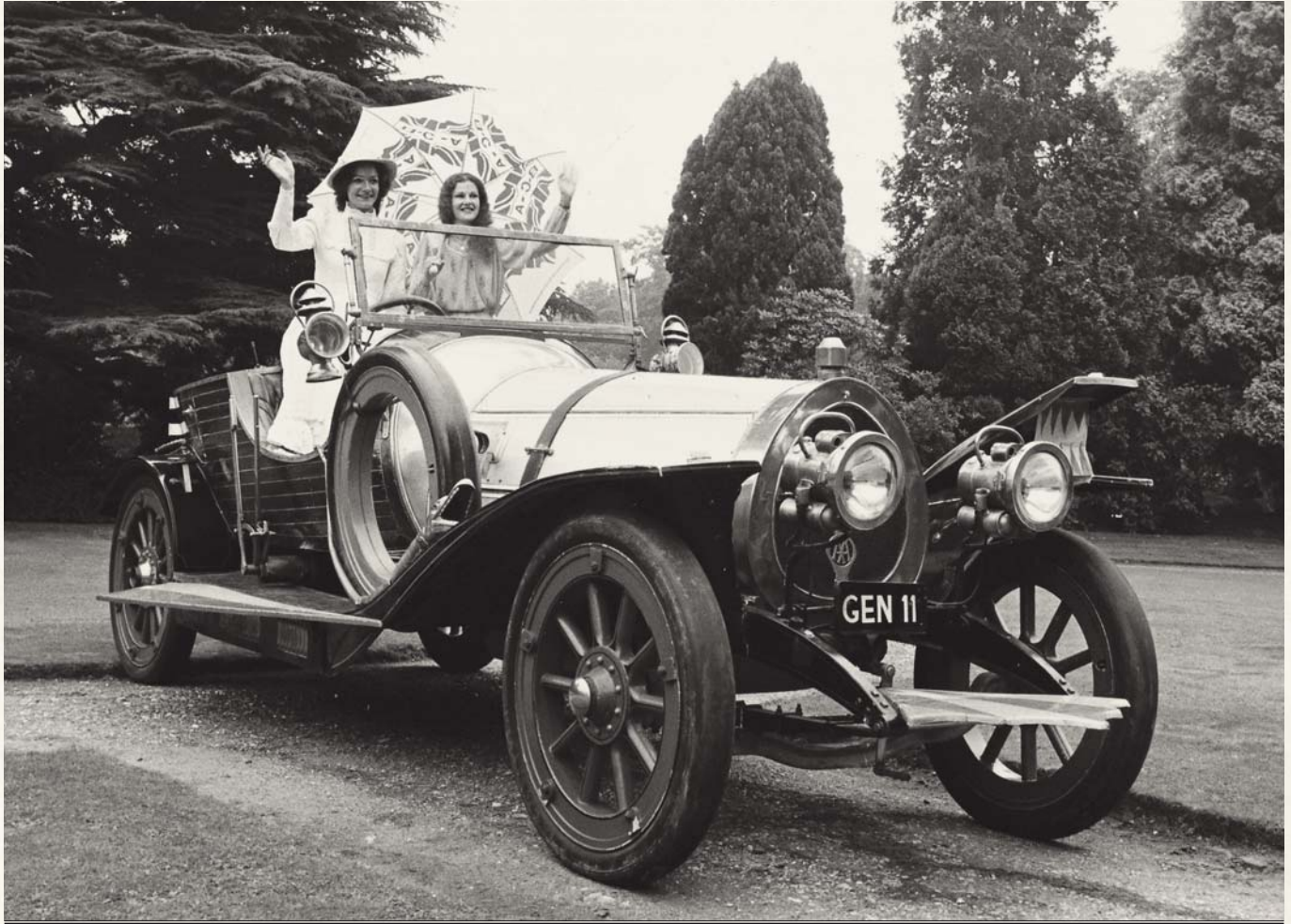
You'd never guess there was a modern Ford V6 engine under that vintage-style hood, and nor that those "wooden" wheels were cast aluminum.
