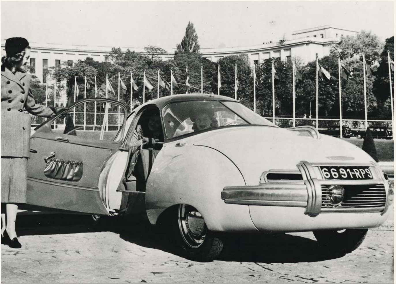
The Panhard Dynavia was outstandingly aerodynamic and amazingly fast bearing in mind the tiny size of its two-cylinder engine.
