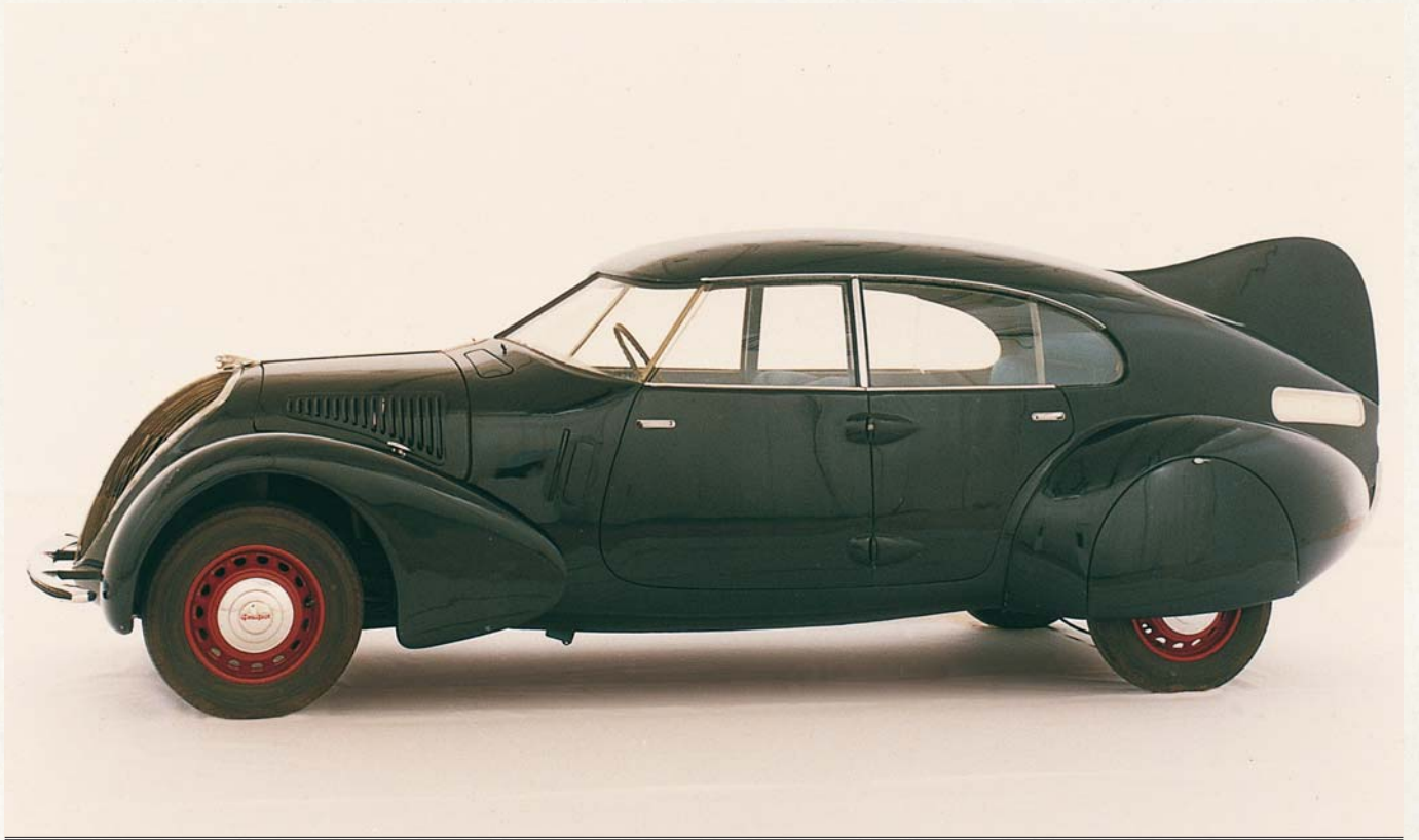
N4X, one of six experimental Peugeots built to test the limits of streamlining for family cars in the near future—which, then, was the 1940s.
