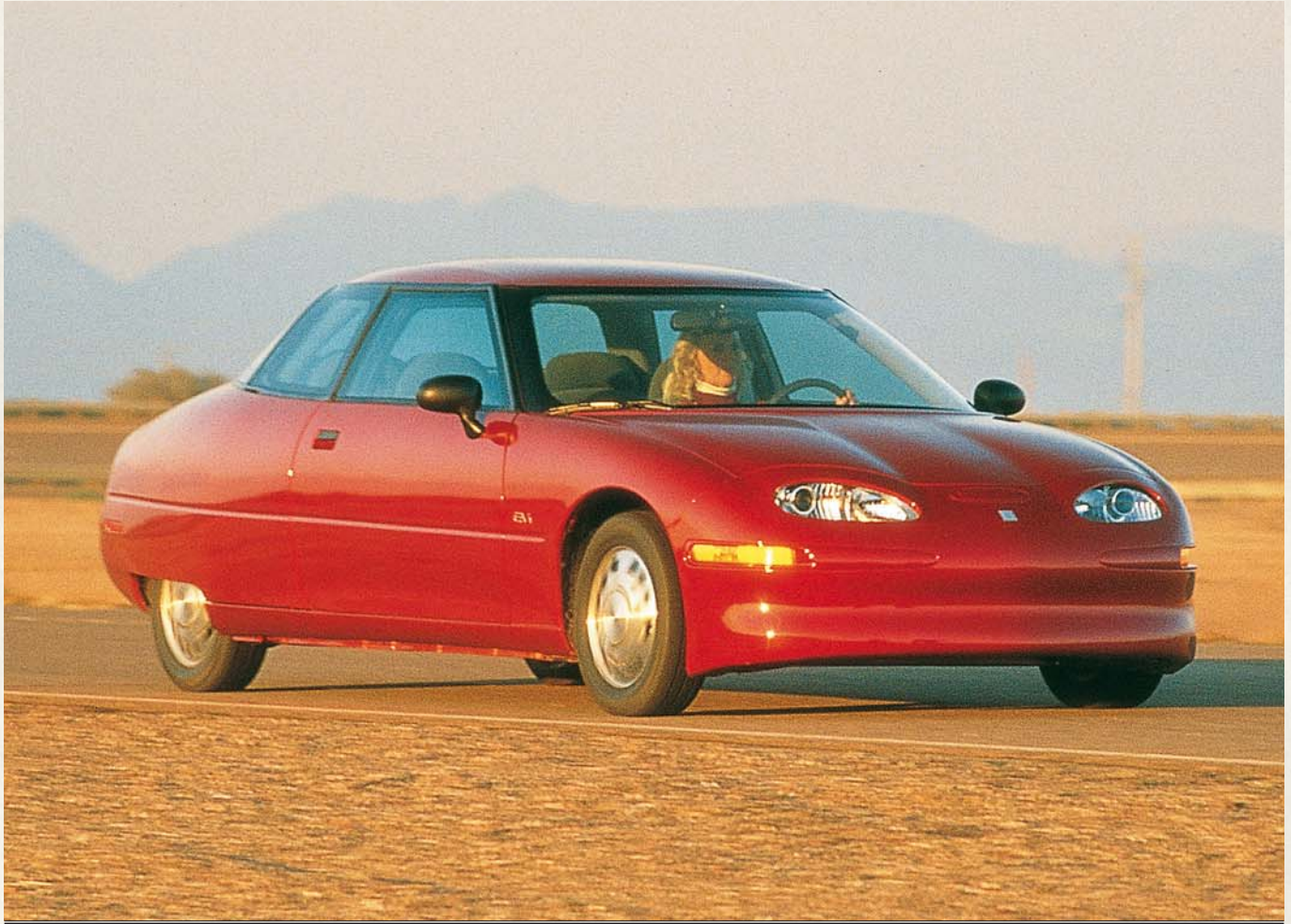
The EV1, with a drag coefficient of just 0.19, is the world's slipperiest production car; this special four-seater model remained a one-off.
