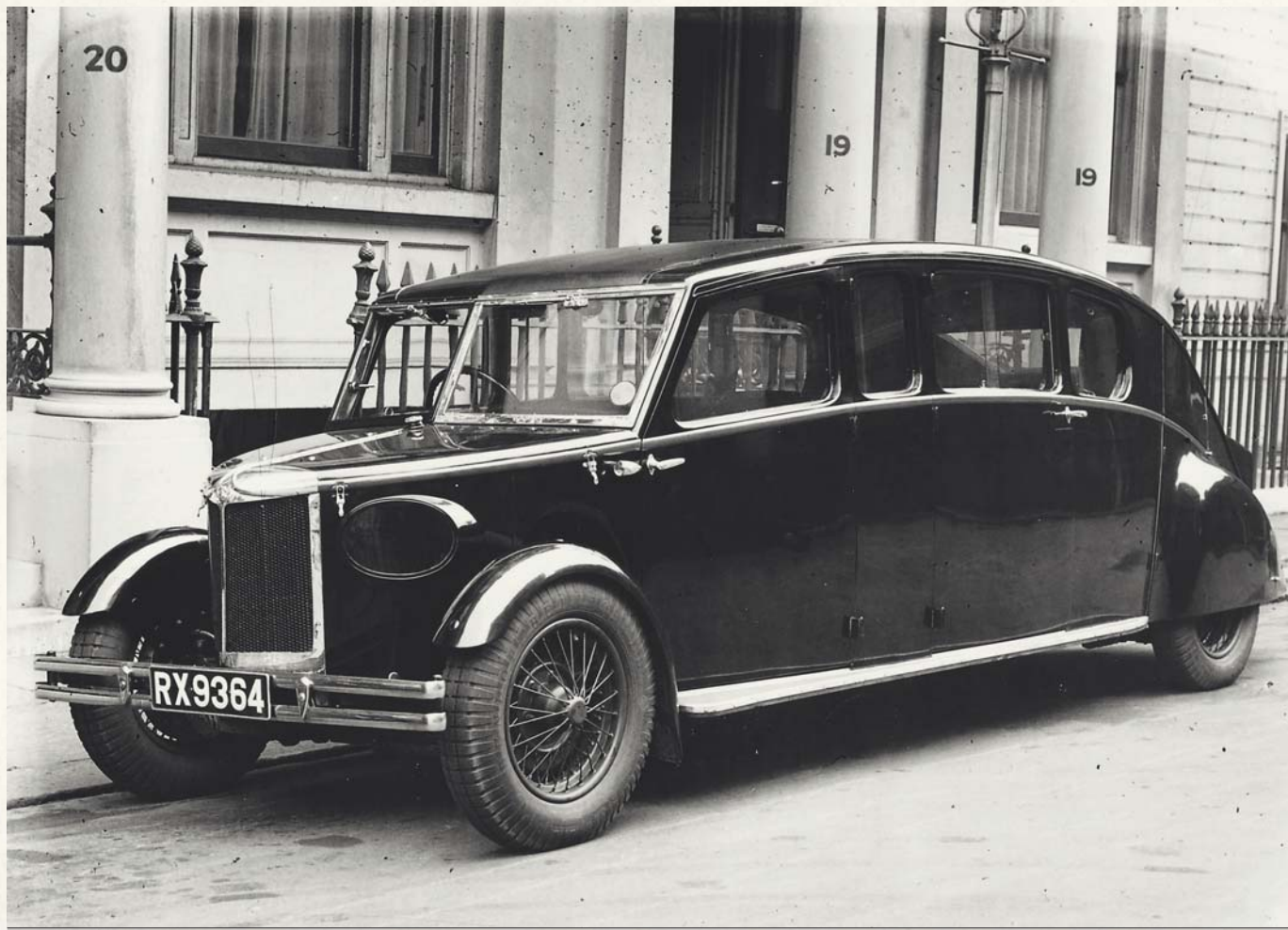
Don't be deceived by that radiator grille—it's a fake. The Burney Streamline's engine was in its tapering tail and, regrettably, prone to overheating.
