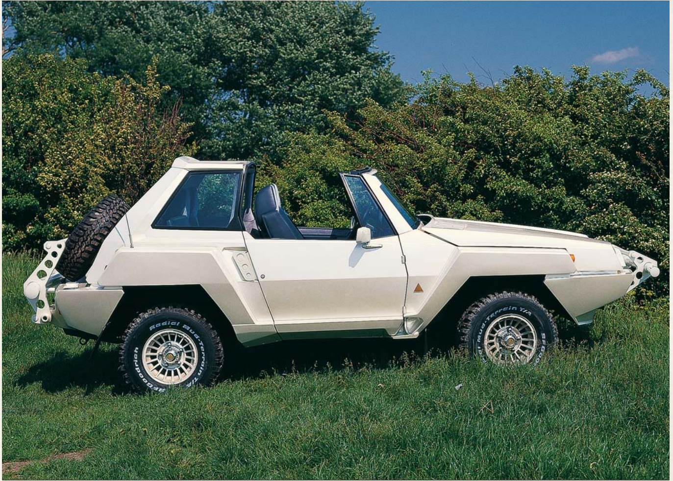
Besides its extremely unusual lines, the Facet offered a removable roof panel that could be stored under its electrically operated hood.
