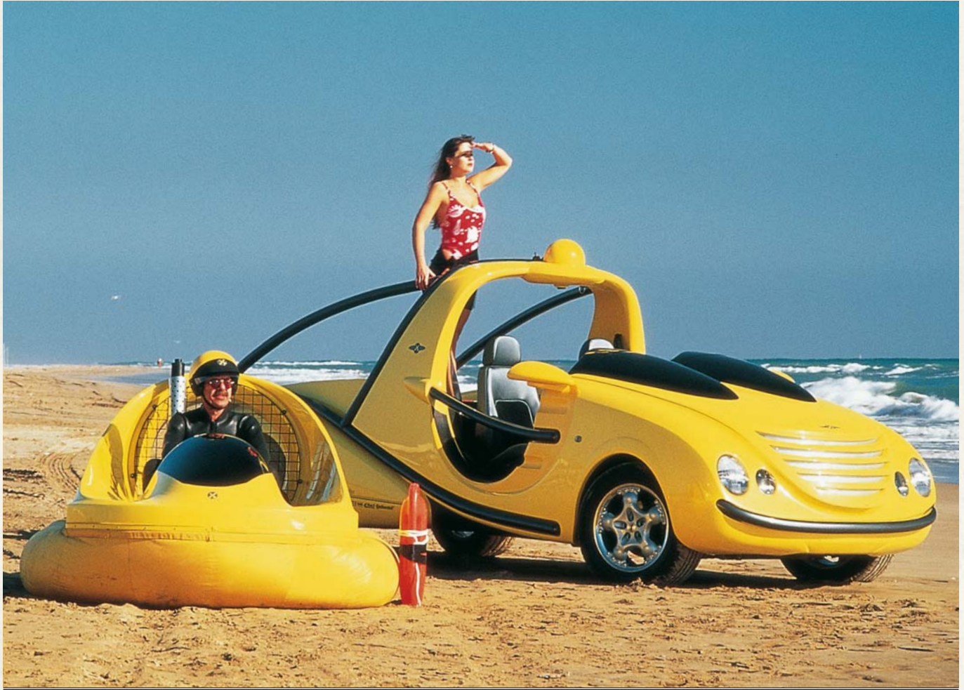
The lifting gear of the X-trem could hoist and deposit its hovercraft and act as a rollover bar if the radical workhorse flipped over.
