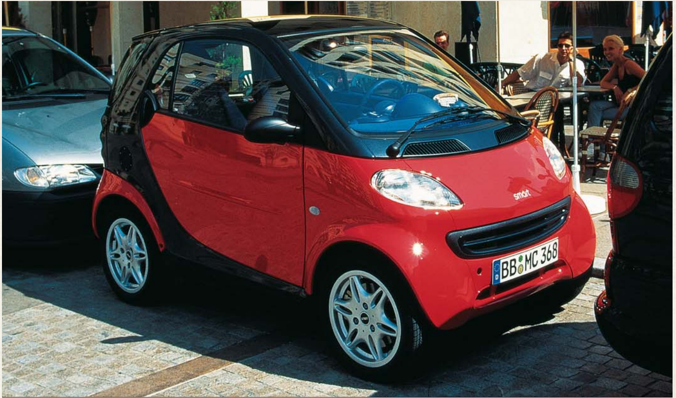
The black body sections of this Smart are its Tridion safety cell, while the red areas are the interchangeable panels as envisaged by Nicolas Hayek.
