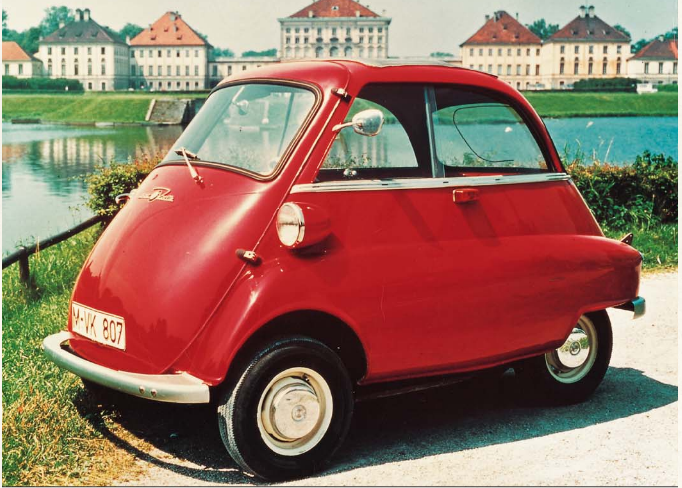
The Isetta's entire front panel swung open to give access to the "bubble" car's interior, while the rear wheels were set a mere 20in (51cm) apart.
