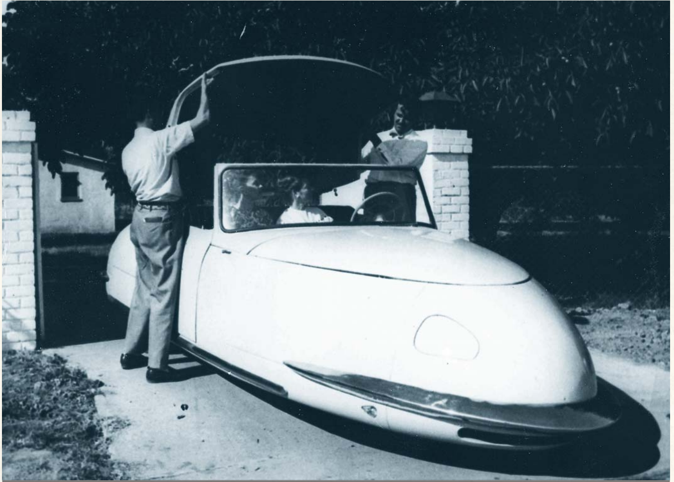
A removable hardtop would have been standard equipment on the four-abreast, three-wheeler Divan, had Gary Davis's ambitious plans succeeded.
