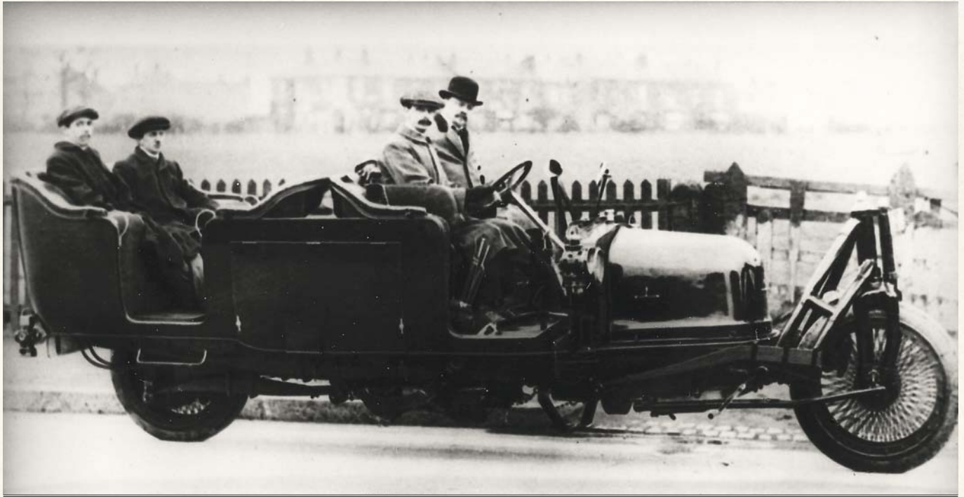
This Gyrocar is standing up on two wheels with four people on board, but its huge turning circle was something of a hindrance when parking.
