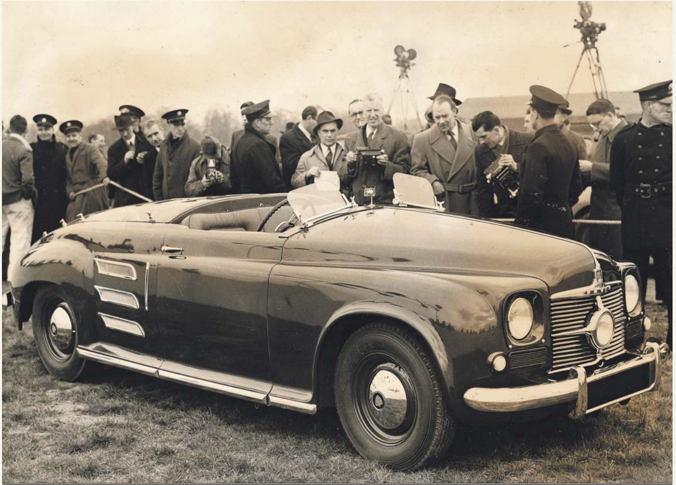
Although similar on the outside to Rover's other catalog products, the large air intakes near the rear wheels hint at the jet power inside.
