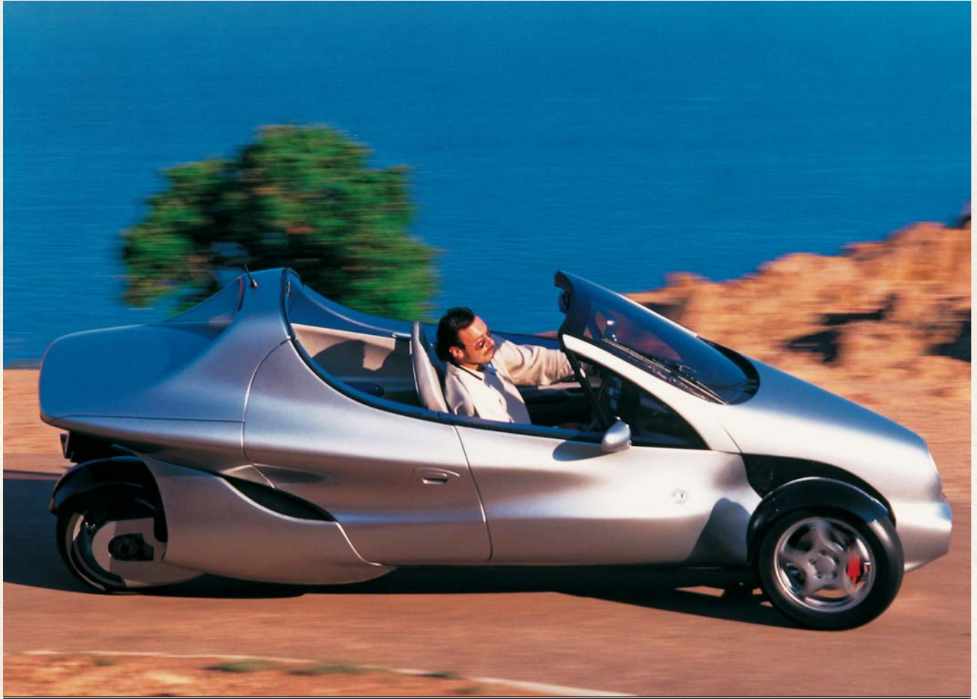
In the back of the Life-Jet was a 98ci (1,598cc) Mercedes A-Class engine powering the rear wheel; the roof could also be stowed for sunny days.
