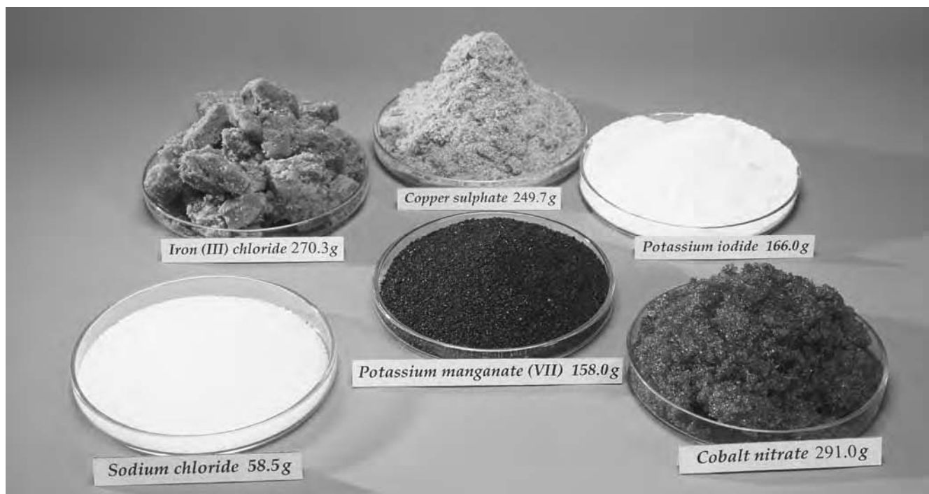
Assorted chemical weights. The different amount of each chemical represents a measurement known as the mole. One mole of any sample contains the same number of molecules or atoms. The weight (shown in grams) of each molar sample is determined by the weight of the molecules (the molecular weight) and is calculated from the weights of the atoms in the molecule. Three of the chemicals are hydrated with water ( \text{H}_2\text{O} ). The chemical formulae are, clockwise from lower left: \text{NaCl} , \text{FeCl}_3 \cdot 6(\text{H}_2\text{O}) , \text{CuSO}_4 \cdot 5(\text{H}_2\text{O}) , \text{KI} , \text{Co}(\text{NO}_3)_2 \cdot 6(\text{H}_2\text{O}) , and \text{KMnO}_4 . The heaviest atom here is iodine (I), eight times heavier than oxygen (O). The transition-metal compounds are colored. (Courtesy of Andrew Lambert Photography/Science Photo Library)
