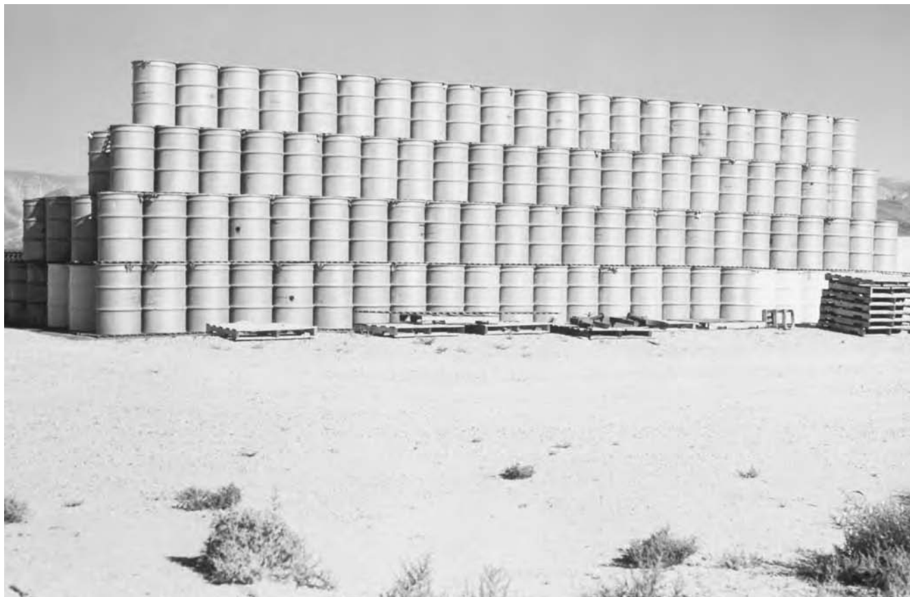
Nuclear waste storage. Steel drums containing nuclear waste at a dump at a nuclear weapons testing site. The drums contain solid waste that is made up of transuranics, radioactive chemical elements with heavy atomic nuclei that are made in nuclear reactions. These drums will be packed, 50 at a time, into steel cargo containers for storage aboveground. Corrosion of these containers will be minimized because of the dry desert climate of the site. Photographed at the Area 5 Radioactive Waste Management Site at Frenchman Flat in Nevada. (Courtesy of U.S. Department of Energy/Science Photo Library)
