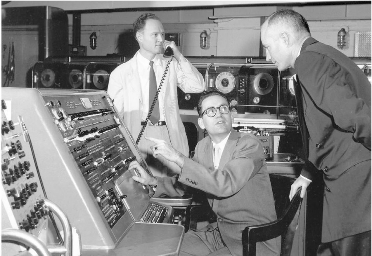
Computing in 1951. U.S. Air Force technicians evaluate the UNIVAC computer system which took up 352 square feet of floor space and ran at a then-astronomical rate of 2.25 megahertz. U.S. AIR FORCE/GETTY IMAGES
