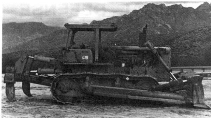
Bulldozer. Note the smoke stack (exhaust pipe).
