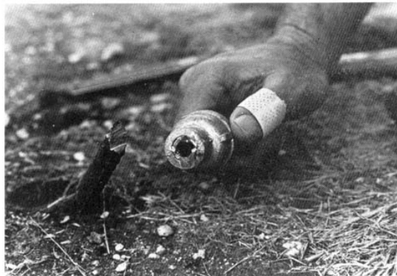
Note the "seat" created in the end of the driver (the 1/4 inch nipple screwed into one of the reducers).
