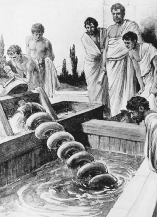
The Greek mathematician and inventor Archimedes oversees a demonstration of his famous screw, a device that raised water from one level to another. TIME LIFE PICTURES/GETTY IMAGES
